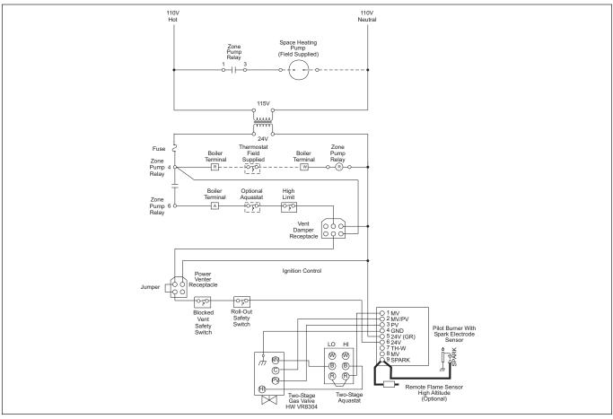
Figure 9f. Schematic, Two-Stage (BJVS 100-225).
